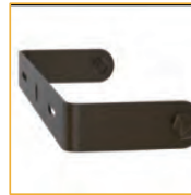
Wall mount adaptor SPCC materials with outdoor powder coating. Code: SP-R11-05a (for 180W,240W and 300W) Code: SP-R11-05b (for 450W,600W )
